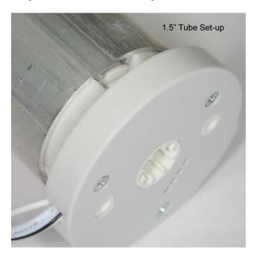
The motor needs to be fully seated in the tube as shown. Push the motor into the tube until the flange of the crown is touching the tube.
