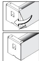
2. INSTALL THE SHADE. Push the clutch straight onto the blade of its bracket. The bottom of the clutch should always point straight down, as shown above. Lower the lug of the end plug onto the V of its bracket. The roller should fit in the brackets securely, with just a little play.
