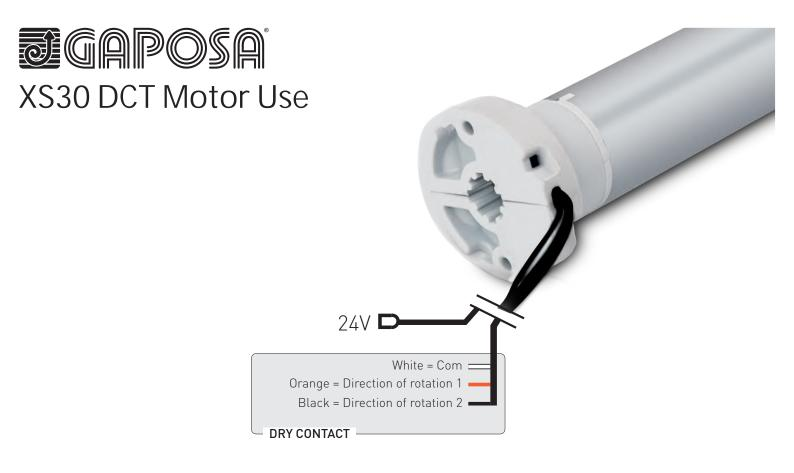
The XS30 motors with both RF and DCT must be programmed via RF remote control. DCT use of these motors is limited to control only. Please refer to the XS30 RF motor programming instructions for motor programming.
